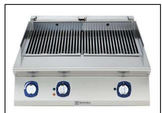
371307 (E7JJCJAOMEG) Full module electric grill top HP (high performance). Heating via incoloy armoured heating elements positioned under removable cooking grid, integrated water tap, fixed well with drain, heat boost deflectros, WRAS - marine
